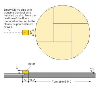
\* Optionally, the motor can be mounted at a larger distance (up to max. 1000 mm) – at an extra charge.
