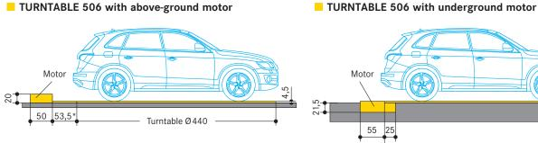
\* Optionally, the motor can be mounted at a larger distance (up to max. 1000 mm) – at an extra charge.
